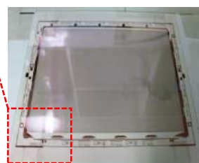
A glass substrate for passive matrix LCDs
